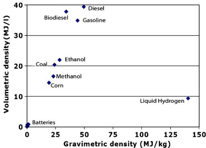
Fig. 1. Caloric energy density of batteries and liquid fuels, (Chu, 2008) according to Eq. (1).
