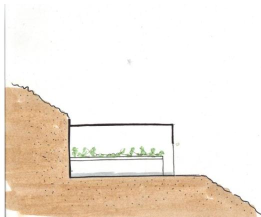
Figure 2: building greenhouse into side of a hill
